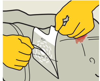
3. Grip tab and peel to remove Foxseal vented from clear liner to expose the adhesive side
