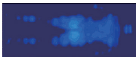
Pressure mapping under Alternating Low Pressure mode
