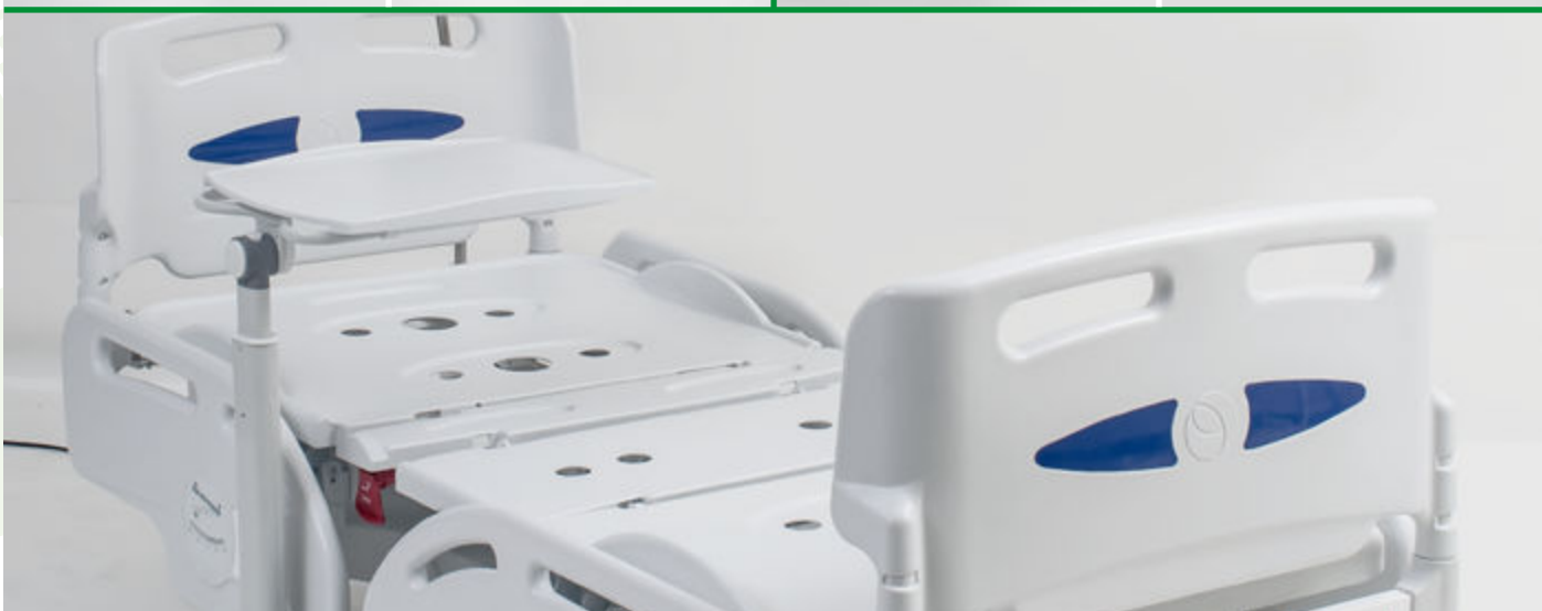
Side table on wheels that can be moved from a place to another. It can be placed near the patient lying surface as the base can be easily inserted under the bed. Functionalities: Interchangeable, swivable, it can be turned according to user's need, tiltable for reading desk, adjustable in height via gas spring. Max load 10kg. Size 420x570mm. Compatible with AC105L.
