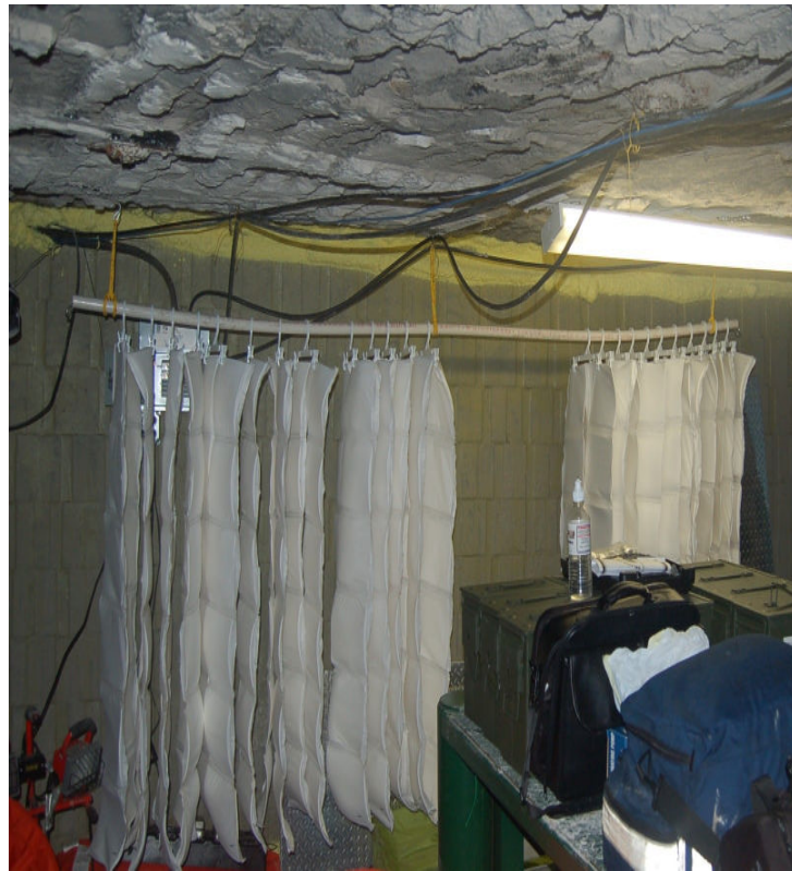
FIGURE 4 DEPLOYED EXTENDAIR® CURTAINS
